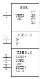
The D+/D- signal pins connect to UTMI pads. The SSTX/SSRX signal pins connect to UPHY and are handled by a single UPHY lane. As UPHY lanes are shared between PCIE, UFS, and XUSB, UPHY lanes must be assigned according to the custom carrier board's requirements.
