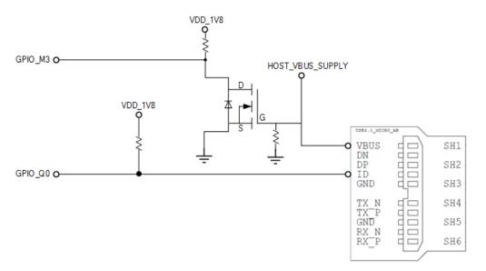
With a B-plug connected, VBUS\_DETECT is logical low, because VBUS is provided from an external power supply, and when no cable is connected it is logical high.
